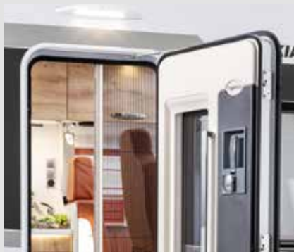
Practical protection: fly screen integrated in the body door
