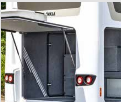
Adjustable rear and side flaps for loading and unloading the storage compartment
