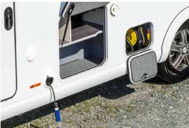
Self-retracting cable reel with 15 m of cable and central supply system
